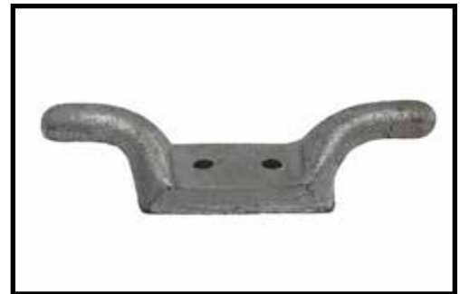
Base is 2-1/2" x 1-1/2" with (2) 1/4" holes on 7/8" centers DC 5AF.....Aluminum Finish
